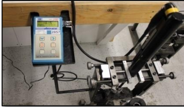
Atlas Copco QST Tool Test
