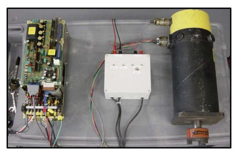
This FANUC velocity control unit (VCU) is a single axis servo control module. This unit is diagnostic tested by a closed loop run / load test with a Fanuc DC servo motor. Also, all VCU I/O points are tested with this fixture. The Fanuc VCU can be either single or dual drive types. Other series units are as listed:
