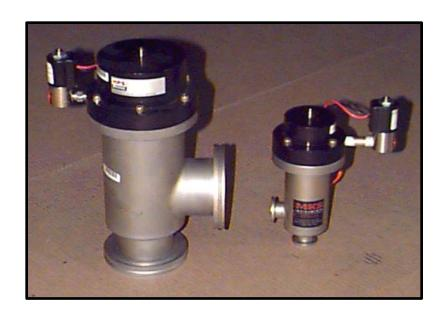
These valves are a High Vacuum relief / control valve. These particular valves are pneumatically actuated as well as using the pressure of the vacuum to move the bellows piston in the unit. They also come in a manual model (not pictured here).
