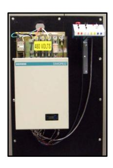
This is the Siemens Simoreg DC drive system. It has been designed to perform full diagnostic testing on the Simoreg drives integral A1-106-100-522 microprocessor regulator control board. Special diagnostic parameters are loaded into this board's memory to ensure that all system functions such as motor control, communications and analog / digital I/O signals operate to OEM specifications. Dynamic run testing on this drive system will ensure a quality repair every time.
