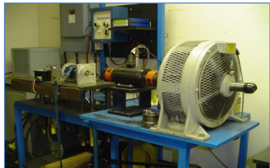
Dynamic load testing on all servo repairs
